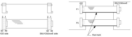
Fig. 5.1.1 External view of the ICE interface cable
